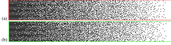
Figure 10: Slices of 3D error-diffusion sampling to a 64 \times 64 \times 256 variable-density volume data. The density changes from 1 to 0 along the z axis. (a) XZ-Slice. (b) YZ-Slice.
