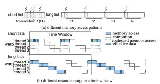
Figure 4: Memory access patterns on lists with different length and concerned time windows
